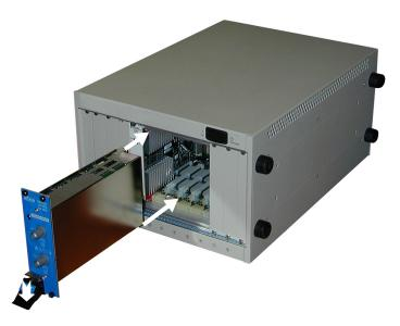
• Power up the chassis. (If you are connecting to the chassis via an MXI-3 connection, power up the computer *after* powering up the chassis.
